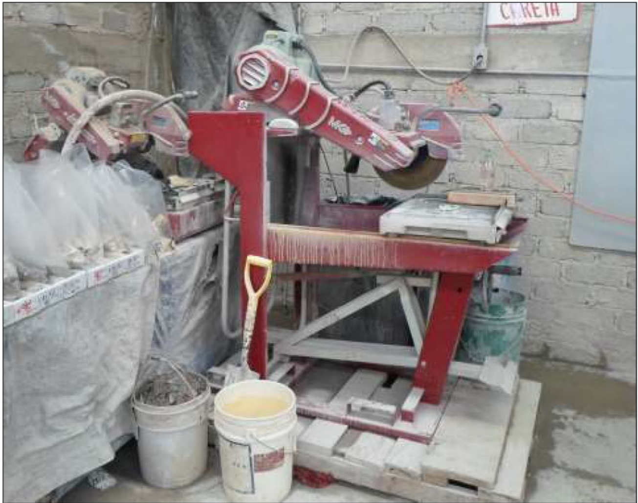
Figure 11.2. One of several core saws located at the exploration core facility Source: National Instrument 43-101 Technical Report: Updated Mineral Resource and Reserve Estimates for the El Cubo Project, Guanajuato State, Mexico for Endeavour Silver, by Hard Rock Consulting, LLC. Effective Date, December 31, 2016, Report Date: March 3, 2017, Amended Date: March 27, 2018.
